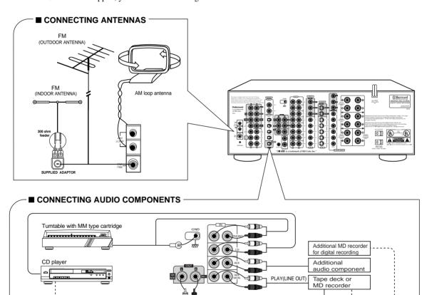
• The AUX jacks may be connected to an additional audio component such as a CD player, a tape deck, etc.
